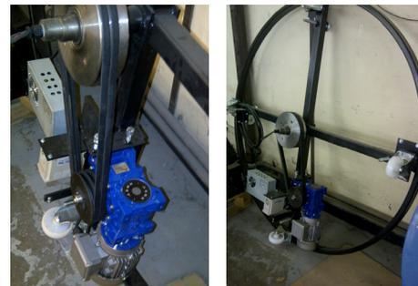
Helical geared motors, **H Series**, size 050 with 2 reduction stages, are used for twist drop towers applications, where the movement speed is not constant and with high torque peaks. These gearboxes are characterized by cast iron casing and hardened/tempered gears.
